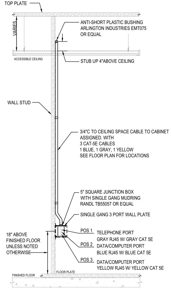
ELECTRICAL CONTRACTOR RESPONSIBLE FOR INSTALLATION OF ROUGH-IN. CABLES PROVIDED AND BY NETWORKING CONTRACTOR. TYPICAL DETAIL - ACTUAL INSTALLATION MAY VARY
