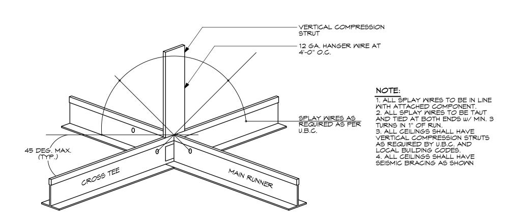
4 SEISMIC CEILING DETAIL
